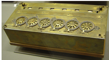
Pascal's mechanical calculator, the Pascaline
