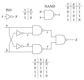
Figure 8.1: The XOR circuit and its components
