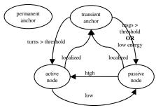
Fig. 2. The automaton regulating the state of a node.
